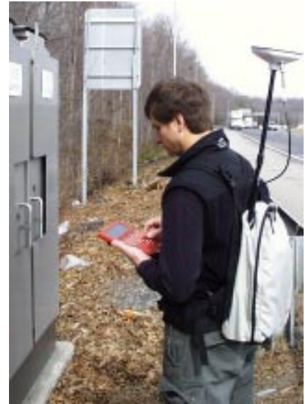
Virginia DOT used a Leica GS50 GPS/GIS unit to record highway signs, traffic cameras, and electrical service panels, along with many other pieces of equipment along state highways.
