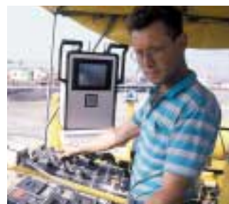
Machine operator Beat Furrer is relieved of control chores by the Leica Geosystems machine guidance system (white box) fitted in the driver's cab – not unlike the aircraft guidance systems which pilots now take for granted. Now he can concentrate wholly on the production process: “Our taxiways are absolutely perfect!”.
