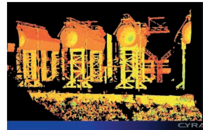
The scanned-in points appear as a "cloud" of variously-shaded pixels, which render individual objects visible.
