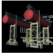
Example Chevron LNG plant: creating an "as built" model of the facility
