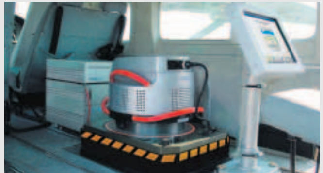
Leica Geosystems' ADS40 is the world's most powerful digital aerial imaging sensor. It records the landscape and its objects for environmental and cartographic purposes with a ground pixel resolution of 15 centimeters. A total of ten channels include infrared and forward, lateral and rear views for three-dimensional interpretation.
