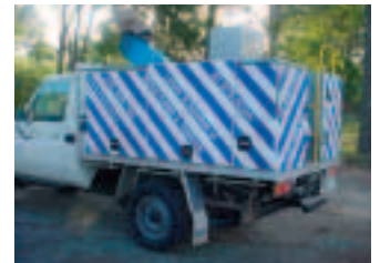
North Surveys have designed a special truck where the cyra laser scanner is mounted on an extendable mast.
