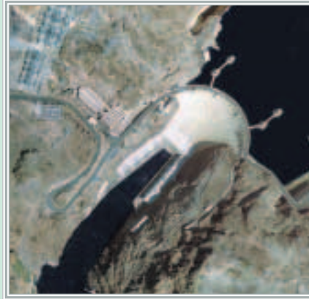
Kenney Aerial Mapping used SOCET SET digital photogrammetric software to create color digital orthophotos of Hoover Dam.
