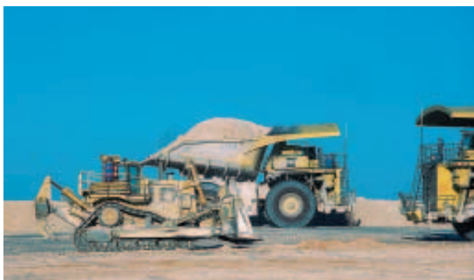
The Leica Dozer 2000T guides and verifies earth-grading by real time GPS.
