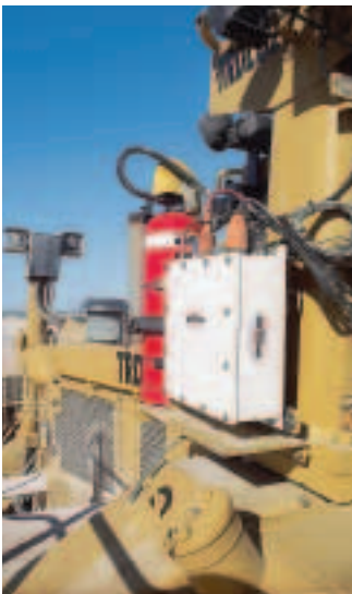
The Leica Dozer 2000T communications components are mounted outside the cab.
