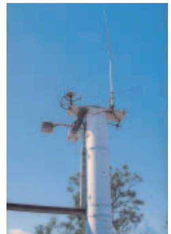
The GPS Base station transmits data to the Rover.
