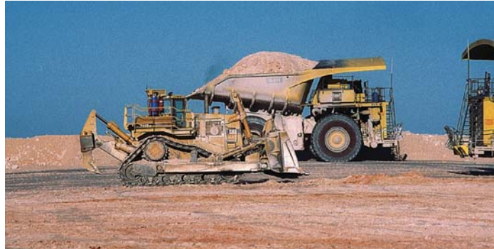
The Leica Dozer 2000T system guides and verifies earthgrading by real time GPS
