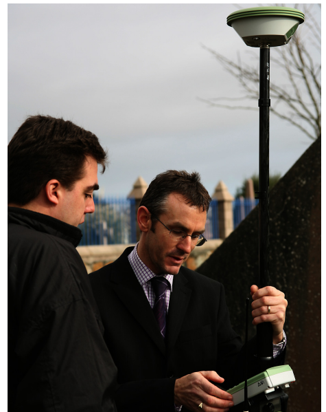
Ben Carruthers of Leica Geosystems training Peter Redmond of Jersey Water to use the Leica SmartRover RTK GPS.
